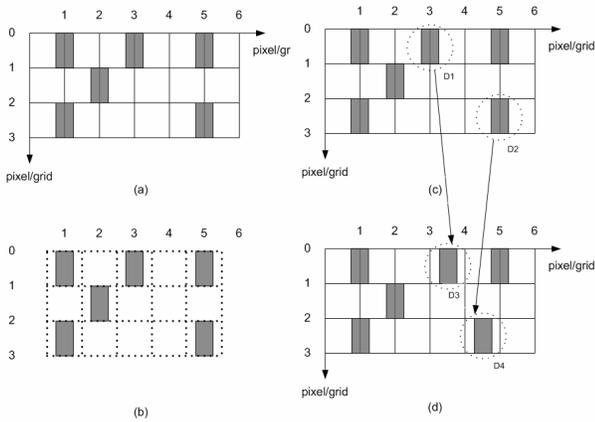
**Figure 1.** Example of (a) halftone pattern, (b) underlying lattices in halftone pattern, (c) halftone pattern before embedding information, and (d) halftone pattern with embedded information.
