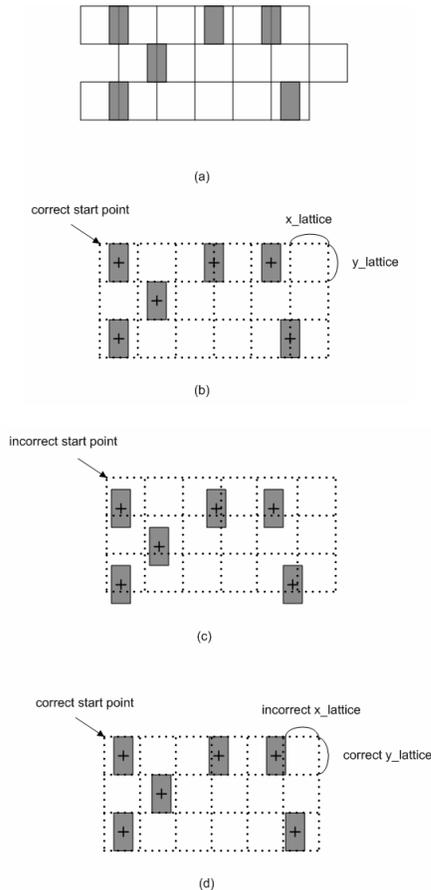
**Figure 4.** Example of (a) halftone pattern, (b) underlying lattices in halftone pattern, (c) halftone pattern before embedding information, and (d) halftone pattern with embedded information.
