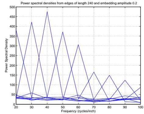
Figure 5. PSDs for each frequency embedded with amplitude 0.2
