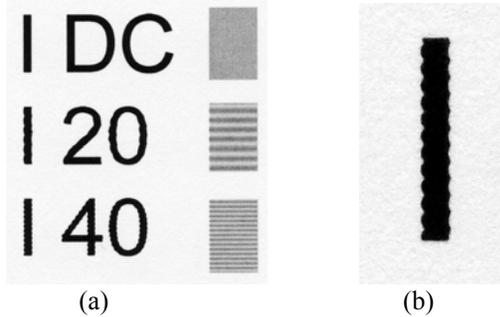
Figure 2. (a) Demonstration of exposure modulation in different images. (b) Magnified letter I in the third row of (a)
