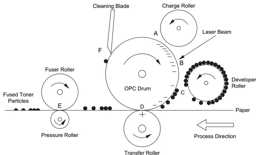
Fig. 4 – Diagram of the EP process.
