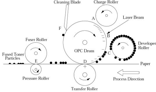
Figure 1 Electrophotographic process: cross-section of a typical laser printer (A) charging, (B) exposure, (C) development, (D) transferring, (E) fusing, and (F) cleaning.
