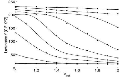
Figure 6 Mapping between reference voltage and luminance of printouts with various default gray values from 10% through 100%
