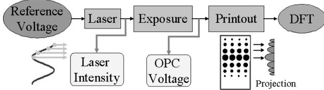
Figure 2 Process block diagram for embedding and detecting extrinsic banding signature using laser intensity modulation.
