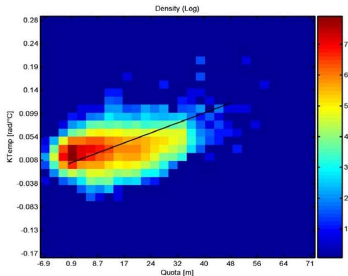
Figure 7. Correlation between PS's thermal dilation [rad/°C] and their elevation [m]. Black line: composite steel concrete building expected trend of thermal dilation as a function of elevation.
