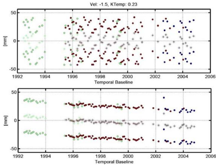
Figure 6. Displacement time series [mm] example. Green dots: ERS-1, red dots: ERS-2, blue dots: ENVISAT. Above: without removing the temperature-dependent term. Below: after removal of the temperature-dependent term. The 2 adjacent replica ( $\pm 28$  mm) are plotted in order to elucidate ambiguities.
