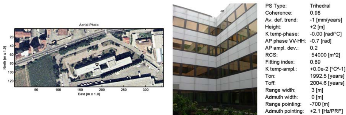
Fig. 8. PS example in Milan: trihedral in a court-yard. Left: aerial photo and PS position. Centre: target photo. Right: list of the PS estimated parameters (height h=2m , high RCS, small L_x=3m L_y=0m , AP phase -0.7rad ).
