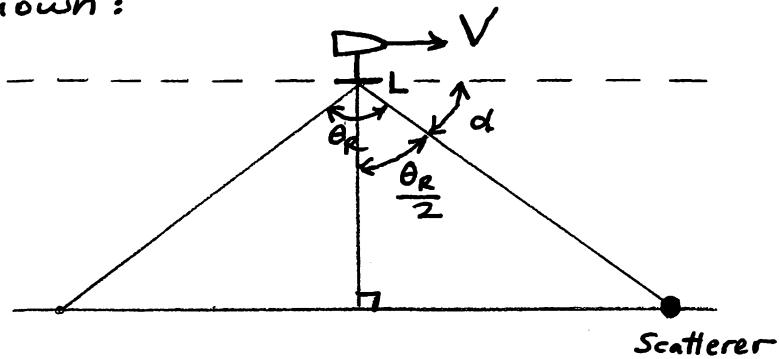
The beamwidth of the real antenna is
