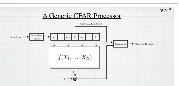
The resolution *cell under test* (CUT) with measurement Y is tested for the presence of the target using a threshold computed using neighboring resolution cell measurements  $X_1, \ldots, X_N$ .
