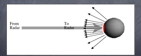
Why is the RCS given by the geometric cross section? The "active area" is smaller.
