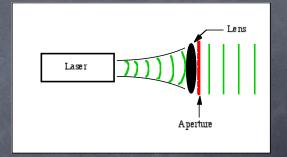
The aperture of an antenna has an area A. This area characterizes the antenna's behavior.
