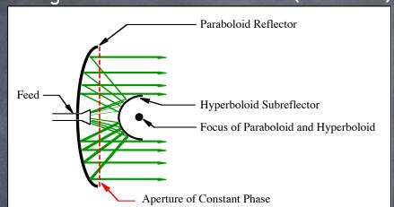
> Path length from Feed to aperture is constant regardless of particular path.
