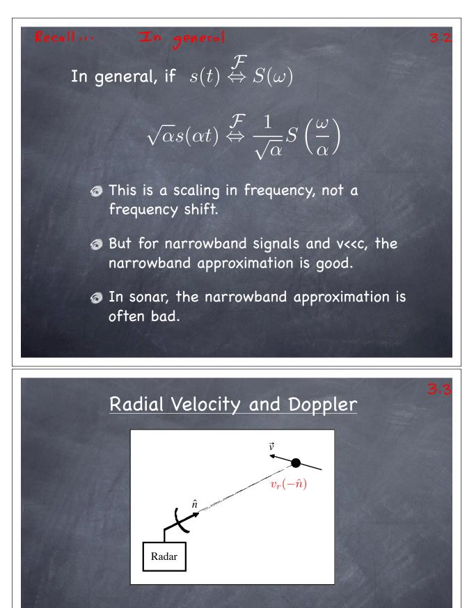
It is the radial component of the velocity that determines the Doppler effect.
