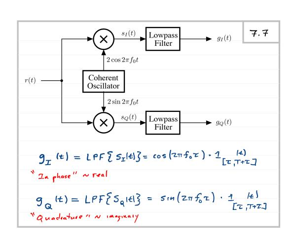
We can construct a complex waveform
