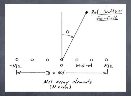
Both arrays have N+1 identical isotropic elements. Elements distributed along line with separation d. Reference scatterer in far-field.
