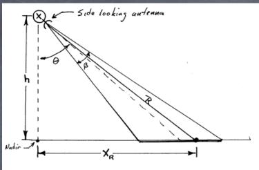
The distance XR can be determined by noting that the range R to the point can be related to Xr by
