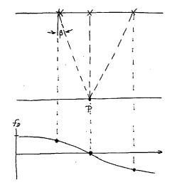
As a radar flies over a target P, the Doppler shift in the signal reflected from P will change at various positions along the path.
