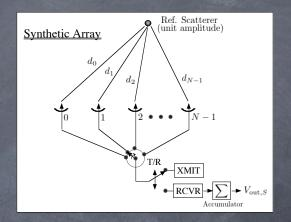
The synthetic array output response is
