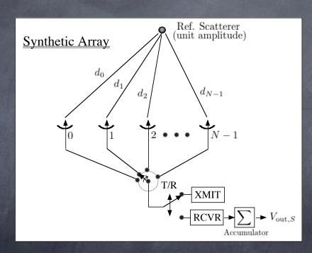
The synthetic array is sequentially built, one element at a time.
