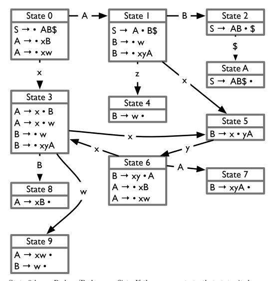
State 9 has a Reduce/Reduce conflict. If the parser gets to that state, it does not know whether to reduce using  $A \to xw$  or  $B \to w$ .
