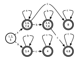
4. Derive the reduced DFA. Show both the graphical representation of the automaton and the state transition diagram.
