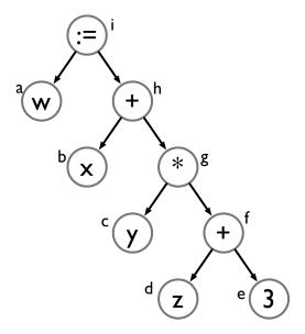
5. Give three address code would be generated for the above tree. Use the following instructions: **LD A**, **T** loads from variable A into temporary T. **OP T1**, **T2**, **T3** performs T3 = T1 OP T2. **ST T**, **A** stores from variable A into temporary T.
