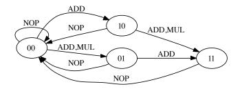
• 2 fully-pipelined resources  $\Rightarrow$  2 bits per state
