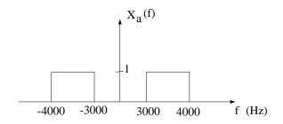
is sampled at a rate  $f_s = 8$  KHz to produce the discrete-time signal x(n), i.e.,  $x(n) = x_a(n/f_s)$ . The sampled signal, x(n), is then input to the discrete-time system below.
