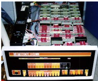
Figure S-3 World’s first “desktop” mini-computer, the PDP-8 (photo by David Gesswein, retrieved from www.pdp8.net ).
