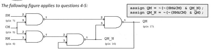
4. The circuit shown above was realized in Lab 8 on a 22V10 using the Verilog assignment statements shown. If the inputs SM, CM, and RM are all set to "1", the outputs QM and QM\_N will be:
