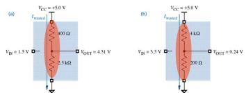
• unused ("spare") CMOS inputs should *never* be left unconnected ("floating") – a small amount of circuit noise can temporarily make a floating input look HIGH (solution: tie unused inputs high or low using a pull-up or pull-down resistor, respectively)
