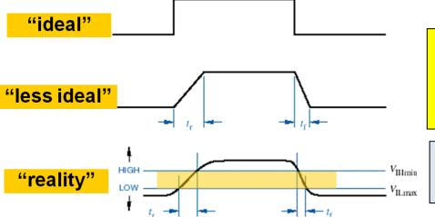
The "name" used for the transition time (t<sub>TLH</sub> vs. t<sub>THL</sub>) is based on what the gate <u>output</u> is doing
