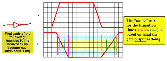
Rise time  $(t_{TLH})$  based on Wakerly's (30%-70%) definition = 2 ns Rise time  $(t_{TLH})$  based on standard 10%-90% definition = 3.5 ns Fall time  $(t_{THL})$  based on Wakerly's (70%-30%) definition = 1 ns Fall time  $(t_{THL})$  based on standard 90%-10% definition = 2.5 ns
