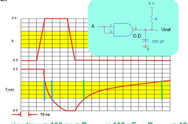
$\label{eq:risetime} \begin{array}{l} \mbox{risetime} = 100 \mbox{ ns = } R_{\mbox{pull-up}} \ x \ 100 \mbox{ pF} \rightarrow R_{\mbox{pull-up}} = 1000 \ \Omega \\ \mbox{fall time} = 10 \mbox{ ns = } R_{\mbox{on}} \ x \ 100 \mbox{ pF} \ \rightarrow R_{\mbox{on}} = 100 \Omega \end{array}$
