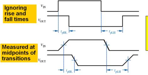
The "name" used for the propagation delay (t<sub>PLH</sub> vs. t<sub>PHL</sub>) is based on what the gate <u>output</u> is doing
