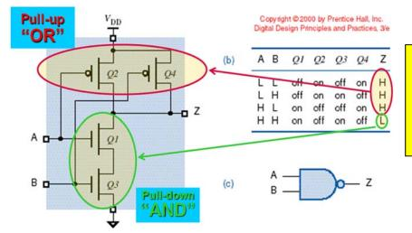
more input combinations pull output high than low → P-channel pull-ups in parallel ("OR"), N-channel pull-downs in series ("AND")
