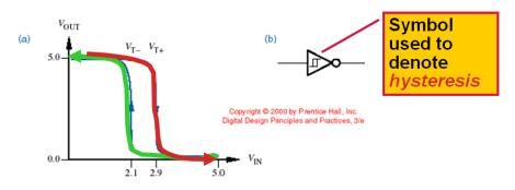
o comparison of Schmitt trigger with regular (single-threshold) inverter
