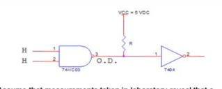
Assume that measurements taken in laboratory reveal that a 74HC03 (open-drain CMOS NAND gate) will produce a  $V_{OL} = 0.2 V$  when sinking +2 mA of current. Also, assume that the  $I_{HL}$  required by a 7404 (standard-series TTL inverter) to recognize a logic "0" is -0.4 mA and that its  $I_{H}$  (to recognize a logic "1") is +40  $\mu$ A.
