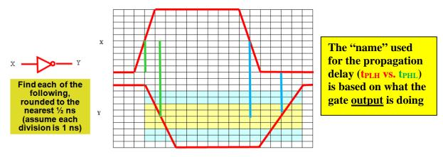
Rise propagation delay  $(t_{PLH}) = 3$  ns Fall propagation delay  $(t_{PHI}) = 1.5$  ns
