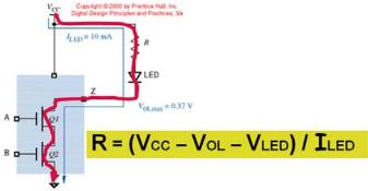
• application - "wired" logic (<u>definition</u>: *wired logic* is performed if the outputs of several open-drain gates are tied together with a single pull-up resistor)
