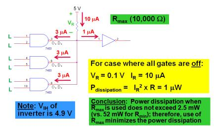
• compare rise time estimates of circuit using R<sub>min</sub> vs. R<sub>max</sub> as the pull-up resistor
