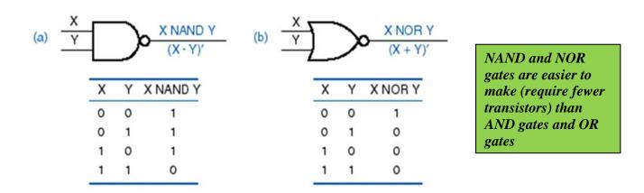
• logical completeness: "anything digital" can be built using solely AND, OR, and NOT gates -or- solely using NAND gates -or- solely using NOR gates
