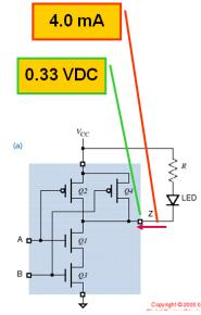
use "Max" value indicated for V<sub>OL</sub> of 0.33 V  $R = V_R/I_{OL} = 2.77/0.004 = 693 \Omega$   $P_R = R \times I_{OL}^2 = 693 \times (0.004)^2 = 11.1$  milliwatts Can also calculate power dissipation of resistor
