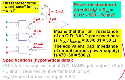
I<sub>OL max</sub> of O.D. NAND gate output: +10 mA @ V<sub>OL</sub> = 0.3 V
