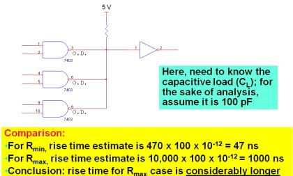
• <u>example</u>: estimate the "on" resistance of an O.D. gate and pull-up resistor value based on rise/fall times
