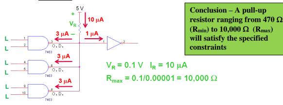
solution, <u>minimum</u> R Value – based on I<sub>OL max</sub> of <u>one</u> gate
