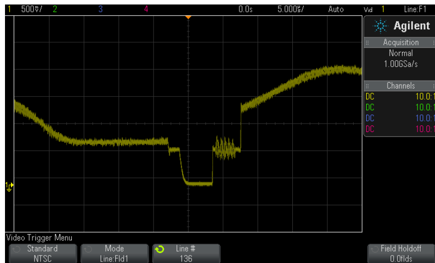
Figure 27 Example: Triggering on Line 136
