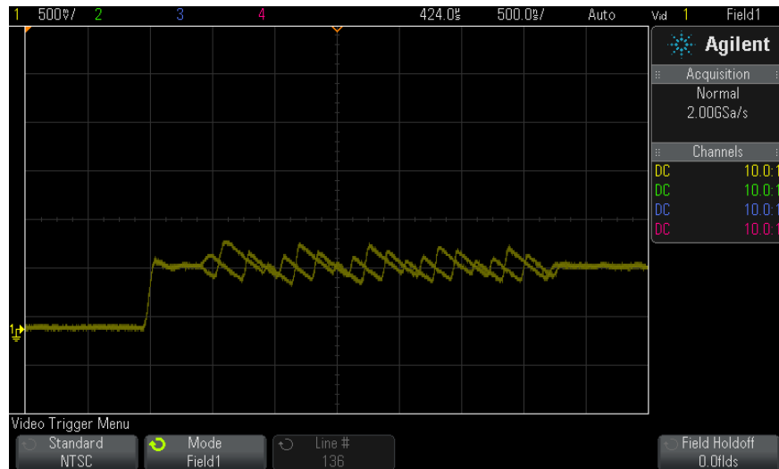
Figure 31 Triggering on Color Field 1 Alternating with Color Field 3
