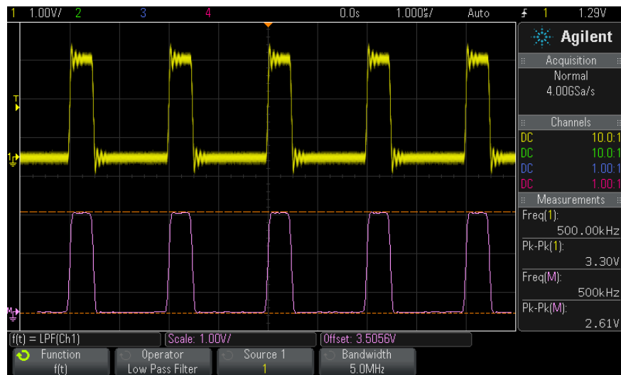
Figure 15 Example of Low Pass Filter
