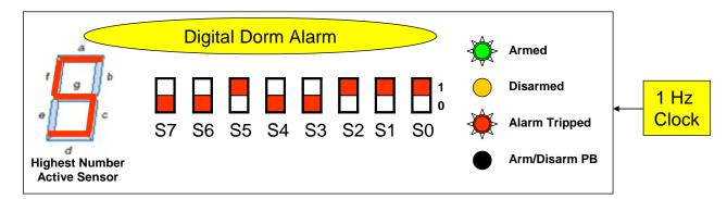
The DDA (Digital Dorm Alarm) in action. The GREEN LED indicates the alarm is in the "armed" state, the blinking RED LED indicates the alarm has been tripped, and the 7-segment display indicates the highest number sensor that is active. The Arm/Disarm pushbutton "toggles" the alarm between the armed and disarmed states. The 7-segment display is *blank* if the alarm is disarmed or, if armed, none of the sensor inputs are asserted.
