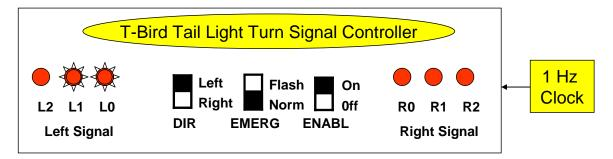
The TBTLTSC taking a *left turn*, for which the output sequence should be: (a) L0, (b) L0 and L1, (c) L0, L1, and L2, (d) all off. This sequence should continuously repeat as long as the enable signal is asserted (ENABL=1). If the "emergency flash mode" is selected, the six lights should alternate between the "all on" and "all off" states (DIR is ignored). When disabled (ENABL=0), all LEDs should be off.
