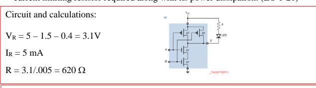
Current limiting resistor =  $620 \Omega$  Resistor power dissipation = 15.5 mW
