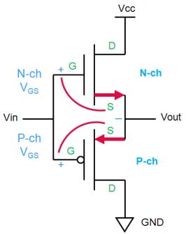
each transistor "flipped" in "upsidedown" circuit → unable to establish V<sub>GS</sub> potential to turn either transistor ON
