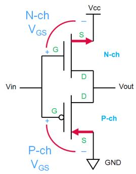
"flipped" upside-down  $\rightarrow$  current unable to flow (cannot pull output high or low)
