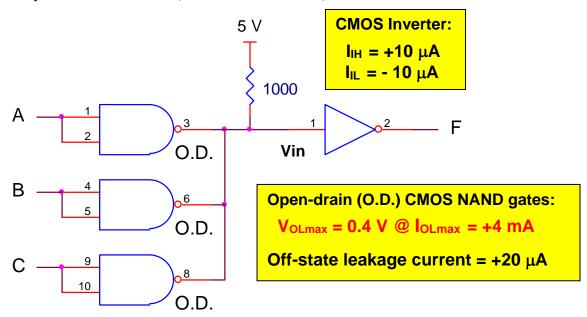
Key: ON resistance of each OD gate is  $0.4/0.004 = 100 \Omega$
