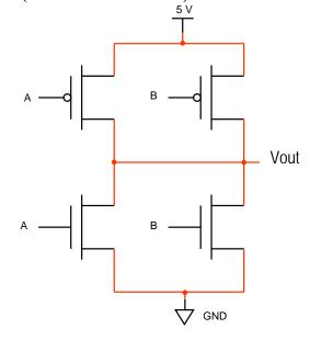
11. A common question students have relates to *why* the P-channel device has to serve as a "pull-up" while the N-channel device has to serve as a "pull-down" (i.e., why can't it be the "other way around"?). To convince yourself of this reality, try drawing a CMOS inverter "upside down" (with an N-channel device used as a pull-up and a P-channel device used as a pull-down) and analyze the circuit you have created (i.e., determine its Vi-Vo characteristics). Describe your conclusion. (LO 1-10)
