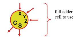
Array should have 4 diagonals/3 rows (12 FA cells total, plus 15 AND gates); worst case delay path is 65 ns
