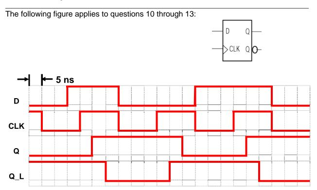
10. The **nominal setup time** provided for the D flip-flop, based on the excitation signals (D and CLK) depicted in the timing chart, is:
