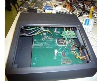
Final Printed Circuit Board (PCB)
