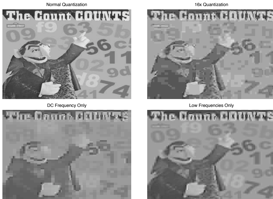
Figure 0.8 Images that were quantized with different quantization levels. Upper left: normal quantization. Upper right: all spatial frequencies were quantized using intervals that are 16 times bigger (4 fewer bits per frequency). Lower left: DC term transmitted, higher frequencies are dropped (note that the 8x8 blocks are now visible). Lower right: only DC and first frequency (a linear slope) are transmitted (note that the 8x8 blocks are no longer clearly visible)
