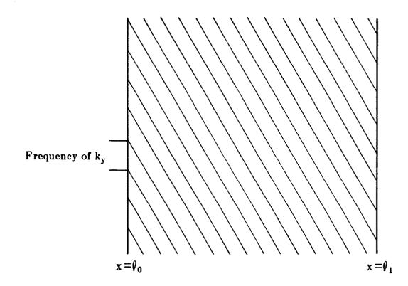
Figure 2.1 A plane wave with direction cosines  $(\sqrt{k_0^2-k_y^2},k_y)$  is shown propagating between the lines  $x = l_0$  and  $x = l_1$ .
