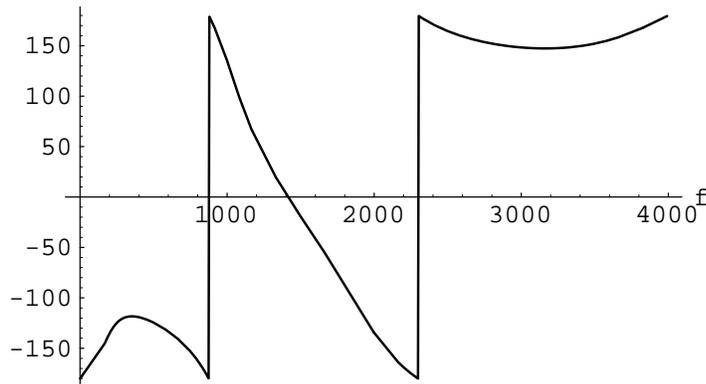
The bilinear z-transform is an alternative to the impulse invariant, or standard-z, transform. The impulse-invariant technique endeavors to match the impulse response of the original analog filter. But there is no guarantee that the impulse response is bandlimited. In fact, there is usually significant energy above the Nyquist frequency which aliases and corrupts the frequency response. Thus the impulse response will be “correct” but the frequency response is wrong.
