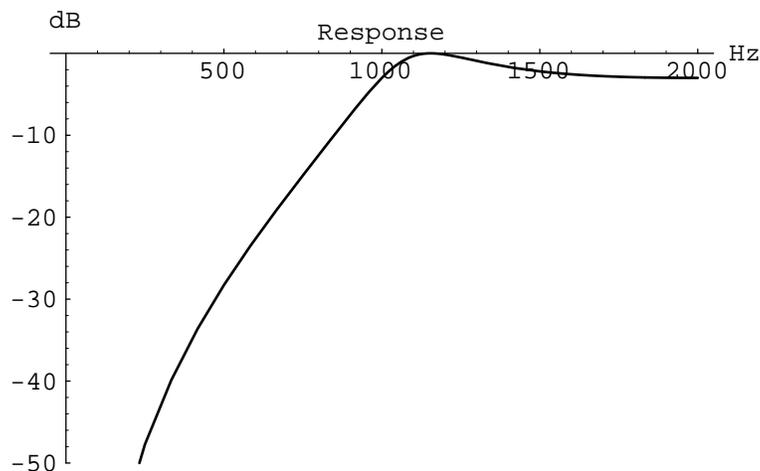
Bandpass filters are more difficult to design. A low pass filter is transformed into a bandpass by specifying the location of the two corner frequencies. We make this transform by substituting the following expression for  $s$  into the normalized low pass filter
