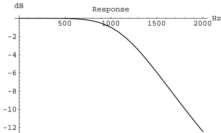
Now we can compare the Butterworth response with a similar filter designed using the Chebychev polynomials. Note that by rearranging the positions of the poles we have designed a filter with a much sharper cutoff. The Butterworth filter has an attenuation of 12dB at 2kHz while the Chebychev filter is already down 20dB. (But in both cases the asymptotic loss for high frequencies will be a function of frequency to the sixth power or 36 dB per octave.)
