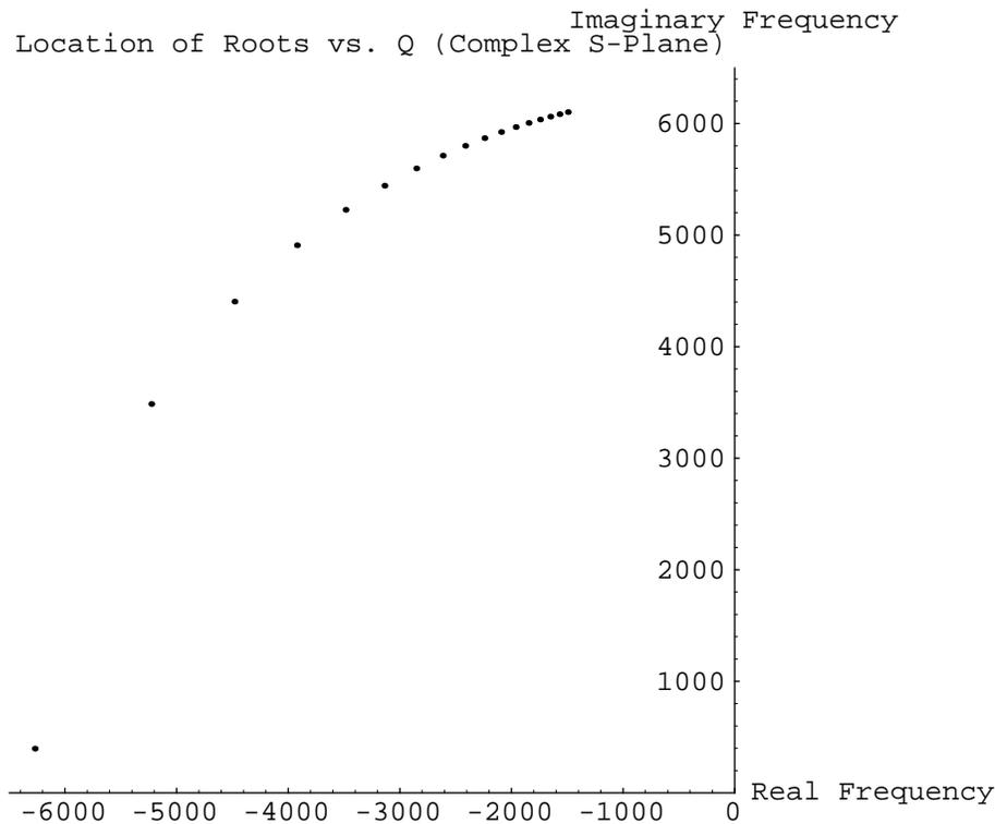
We create a second order filter using a pair of complex conjugate roots as a function of the complex frequency  $s$ .
