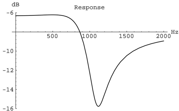
A second filter is shown below. We have combined a broad notch with a narrow resonance to give a bandpass filter.
