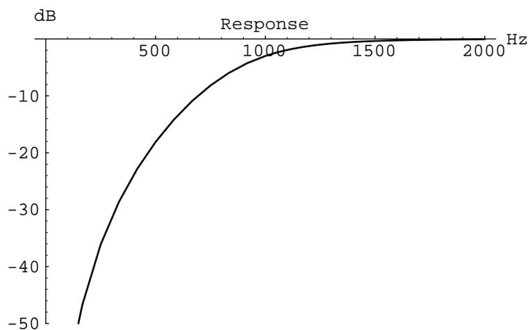
The next example is the normalized third order Butterworth above transformed into a bandpass filter with corner frequencies of 1000 and 2000 Hz.
