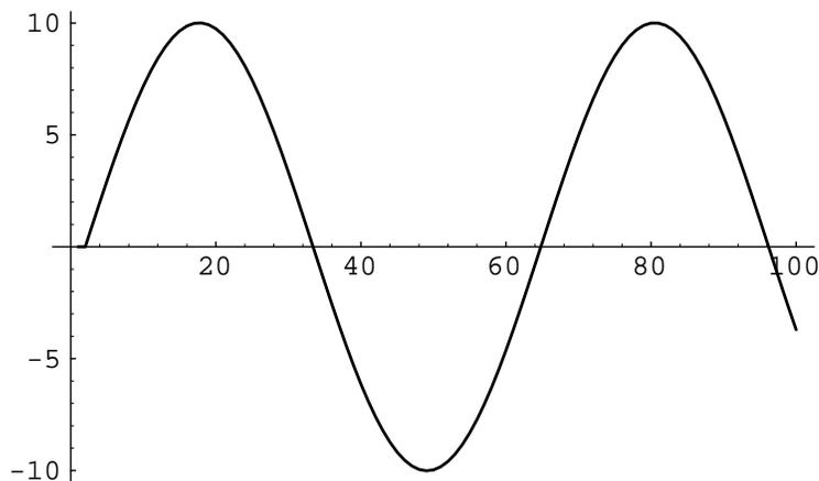
A second order filter with finite  $q$  will have an impulse response that is a decaying sinusoid. The following example shows the impulse response to a second order filter with a center frequency of 1000 Hz, sampling frequency of 8000 Hz and a  $q$  of 10.
