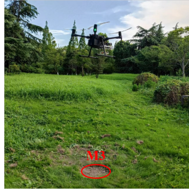
Fig. 30. Radar signal collection and soil moisture measurement at M3 by the UAV-based system.
