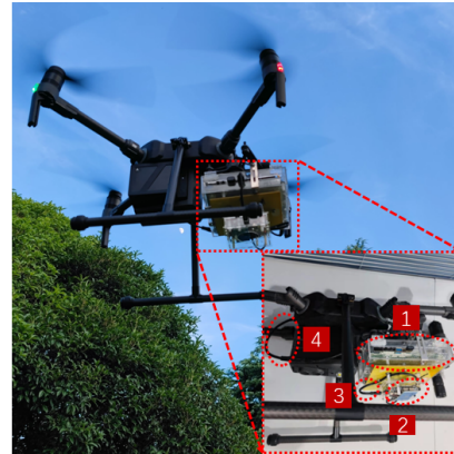
Fig. 10. Overview of the UAV-based system, where the numbered components represent 1: mini PC, 2: IR-UWB radar, 3: power cable from the mini PC to the IR-UWB radar, and 4: power cable from the UAV to the mini PC.
