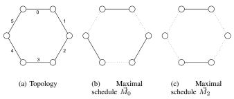
Fig. 2. The 6-link cyclic network and the instances of maximal schedule under the 1-hop interference model. The solid lines in (b) and (c) are the active links.
