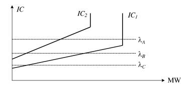
$\lambda\text{-iteration}$  method for two generators with quadratic costs
