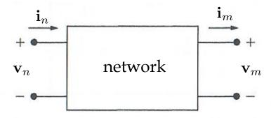
• Matrix generalization of the transmission line model
