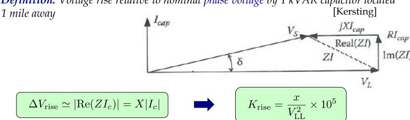
**Example:** For the previous line, find the  $K_{rise}$  and the capacitor rating needed to fix a voltage drop of 3.5% to 2.5% located 1.5 miles away
