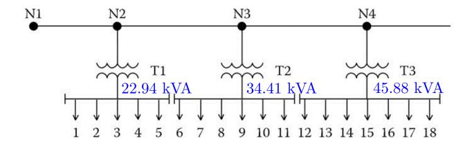
Easier to implement, but good only for voltage drop calculations; since it assumes load has been allocated to XFMs properly
