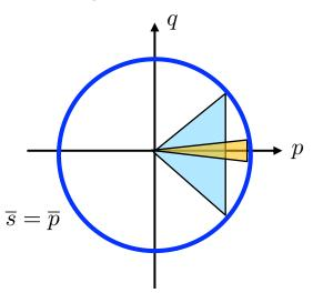
• By oversizing inverters by 10% (kVA=1.1kW), p can be compensated by 45% q even at peak solar
