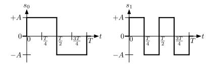
The channel is an additive white Gaussian noise channel with psd height  $N_0/2$ . The Bayes criterion is to be used with equally likely priors, i.e.,  $\pi_0 = \Pr[s_0 \text{ is trans.}] = \pi_1 = \Pr[s_1 \text{ is trans.}] = 0.5$ . Find the average probability of error in terms of A, T,  $N_0$ , and the function  $Q(\cdot)$ . Assume that the receiver has been optimally designed. Explain your work and show any calculations needed.
