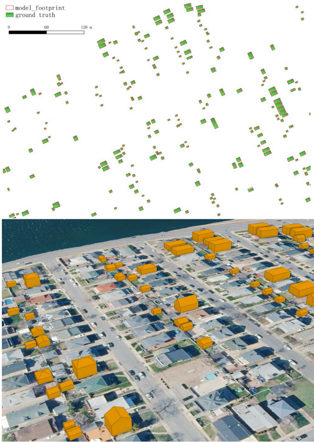
Fig. 11. Footprints (top) of reconstructed models (red) and ground truth (green), and a 3D view of the reconstructed building models (bottom).
