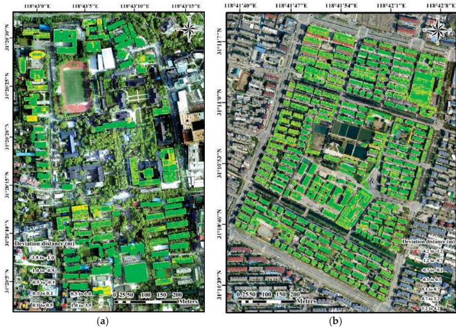
Figure 10. Deviation distances between the reconstructed building roof models and the LiDAR-derived validation data, as represented by points with different colors: (a), (b) Region 1 and Region 2, respectively.
