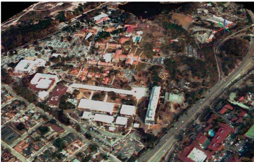
Figure 12. “Fused” HRQLS-1 lidar-photographic 3D image of the Naval Post Graduate School in Monterey, California.
