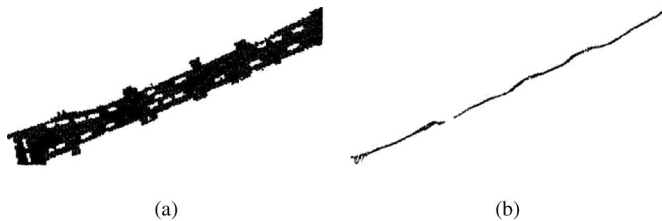
Fig. 3. Mean shift clustering for the detection of road center points with holes in the area. (a) Road points with holes. (b) Clustered mode points by the mean shift.
