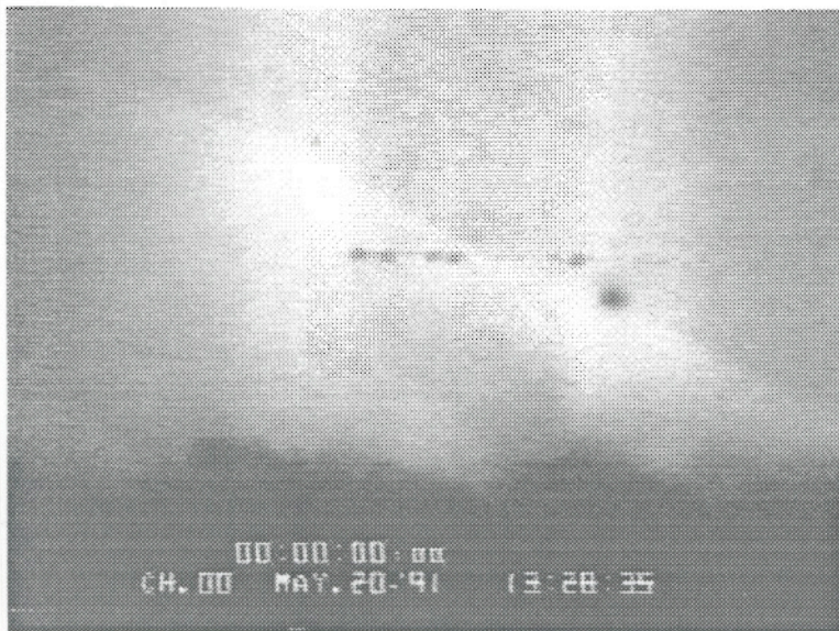
Figure 8: Rayleigh scattering images the flow in the vicinity of separation. (a) undisturbed flow, (b) concentrated blowing.
