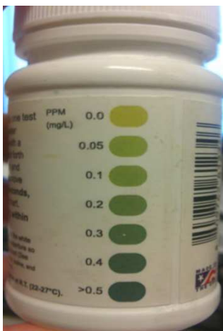
Figure 4. Concentration key on ozone test strip bottle
