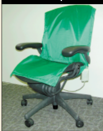
Figure 3. The sensing chair is a haptic PUI
