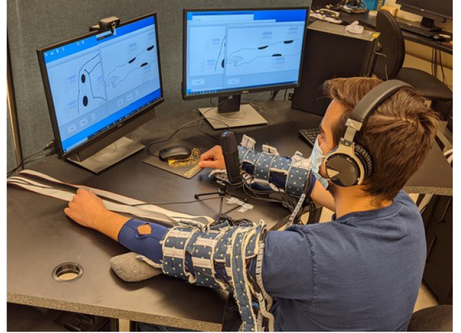
Fig. 7. Photo of a participant wearing one tactile display on the upper left arm and the other on the right forearm (from [14]).
