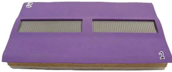
Fig. 8. The test apparatus for holding two stainless steel blocks with surface gratings. The numbers “1” and “2” were used by the experimenter to determine which grating should be presented to the left of the participant on each trial. The apparatus was always obscured by a curtain from the participant’s view.
