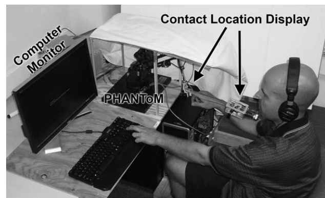
Figure 9. Experimental test setup (cover pulled back for clarity).
