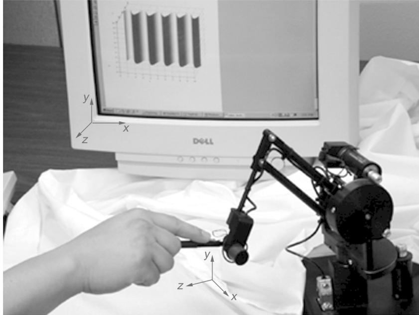
Figure 1. Illustration of experimental set-up. The user held a stylus attached to a PHANTOM force-feedback device (foreground). The textured surface was a sinusoidal grating that varied only along the x-direction on a vertical plane (background, not shown during psychophysical experiments).
