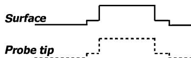
Fig. 1. An illustration of a surface profile (solid line) and the trajectory followed by the probe tip (dashed line) when the surface is explored with a haptic device.
