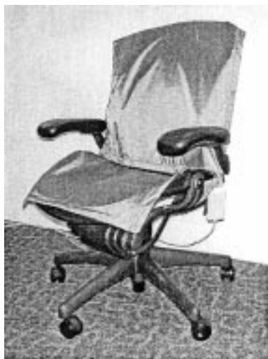
Fig. 1. The sensing chair.
